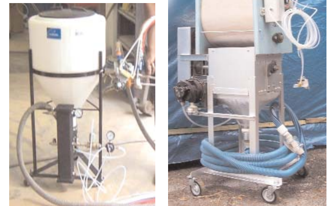
Seawolf's Recycled FRP (above) & Natural Fiber (left) Spray Guns
